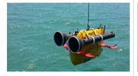
This nimble robot can dive into the deep sea to more than 2000 meters, where pressures can reach a bonecrushing 3150 psil Nicknamed 'PlankZooka', the sampler vehicle has been adopted to collect tiny plankton living near the sea floor without destroying them for scientific analysis. Find out how it works from this Scientific American article. entrepreneurship What's Your Type?
